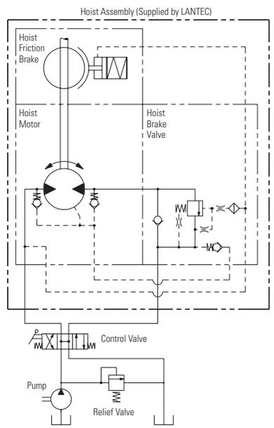
Typical Hydraulic Circuit for 2-Speed Motor
