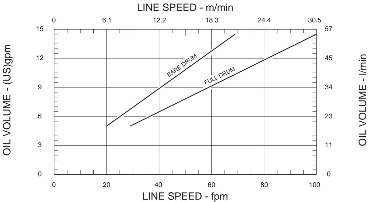
Performance graphs are based on standard hydraulic motor and cable drum with 1/2 inch diameter wire rope.
